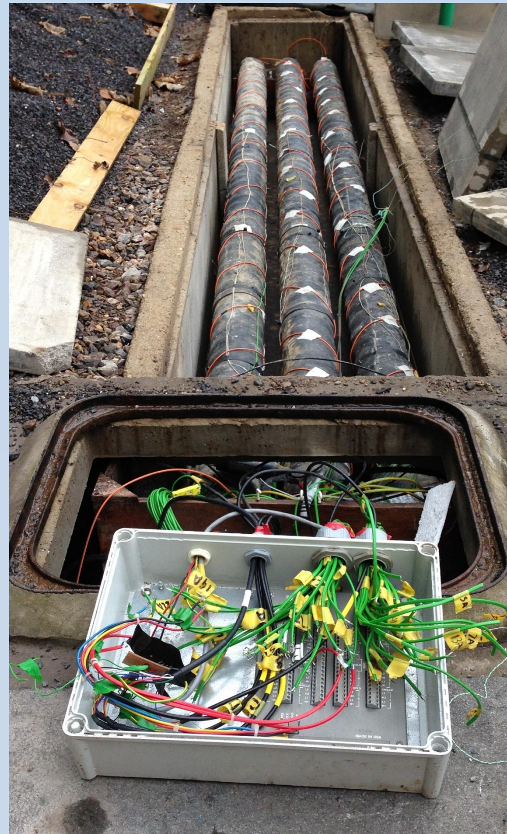
Figure 2 Cable duct test bed for prognostic indicator assessment
