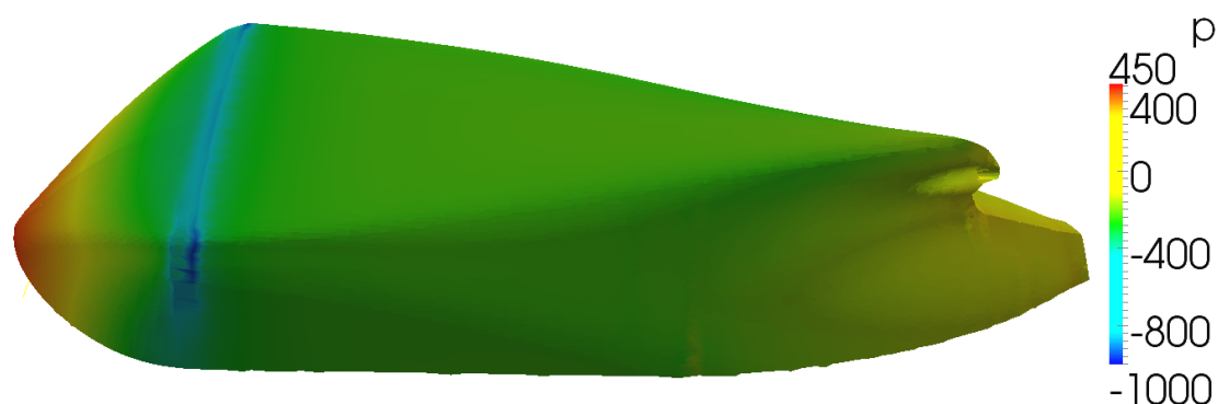
Figure 19: Pressure distribution on hull as predicted by CFD
