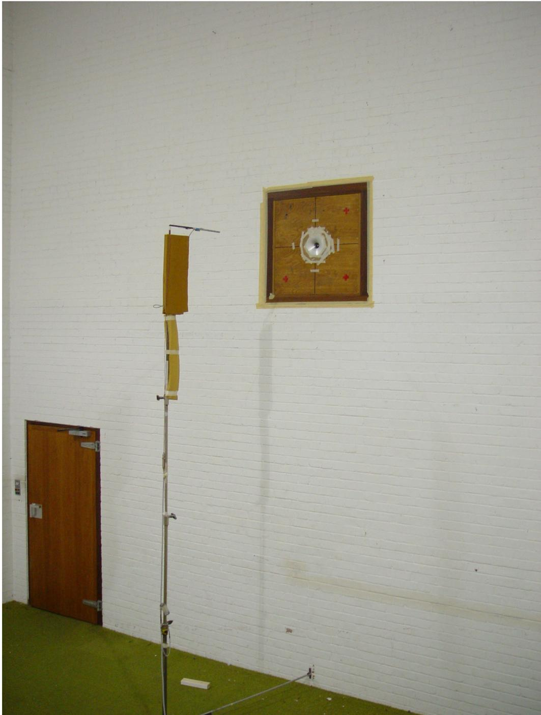
Figure 7.61. Photograph of the Transient Room measurement facility at the KEF Audio (UK) research and development centre. The room measures 20m in all directions. The test horn is visible in the centre of the wall opposite the camera. The microphone is positioned on the tall stand and located mid-way up the height of the room in order to ensure maximum possible window time.
