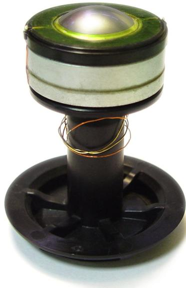
*Figure 7.56. Main tweeter assembly with the phase plug removed.*
