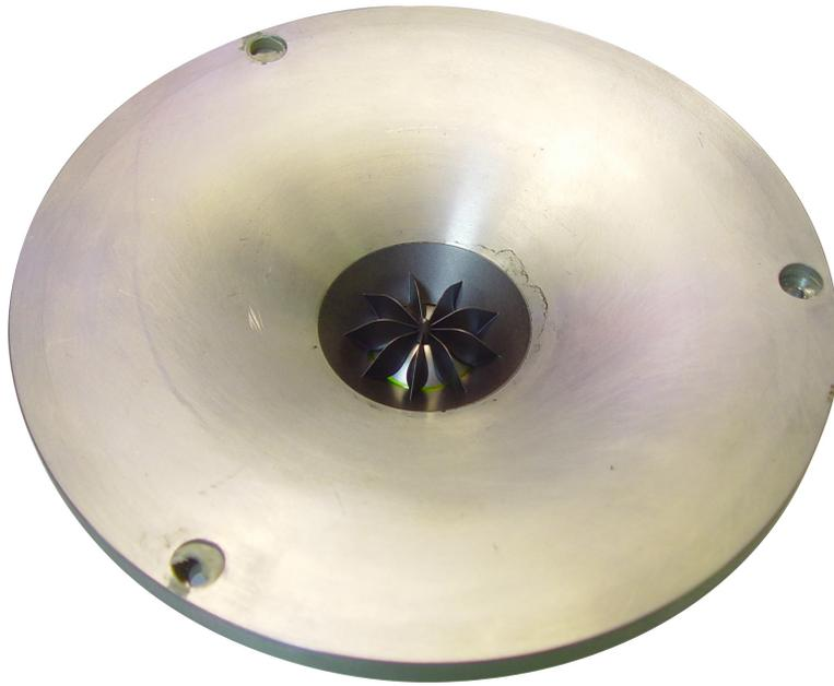
Figure 7.58. Tweeter placed in test horn.
