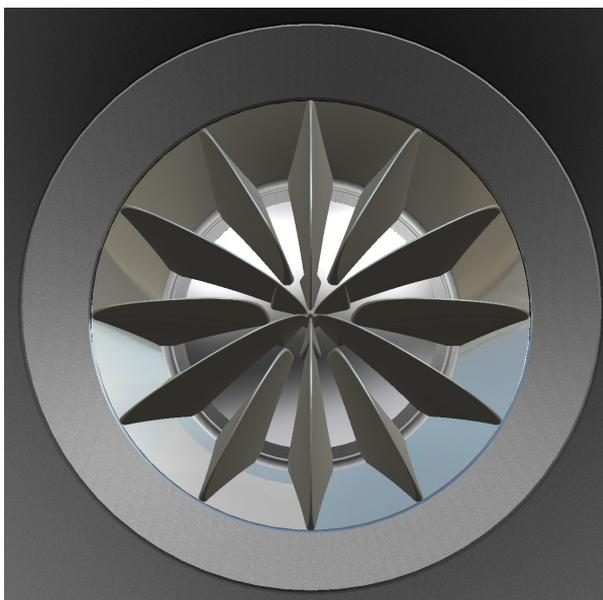
Figure 7.14. 3D CAD rendering of the practical implementation of the  $\cos$  weighted radial-channel phase plug showing inner area with fewer radial channels.
