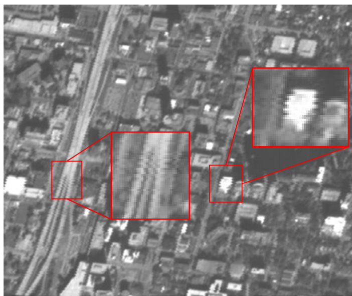
Figure 1-1 Effects of microvibrations on geometric distortions [8]
