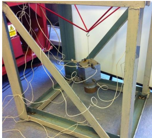
Figure 6-9 WA-seismic mass coupled microvibration test setup
