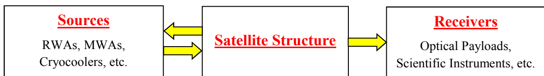
Figure 1-3 Propagation of microvibrations on satellites
