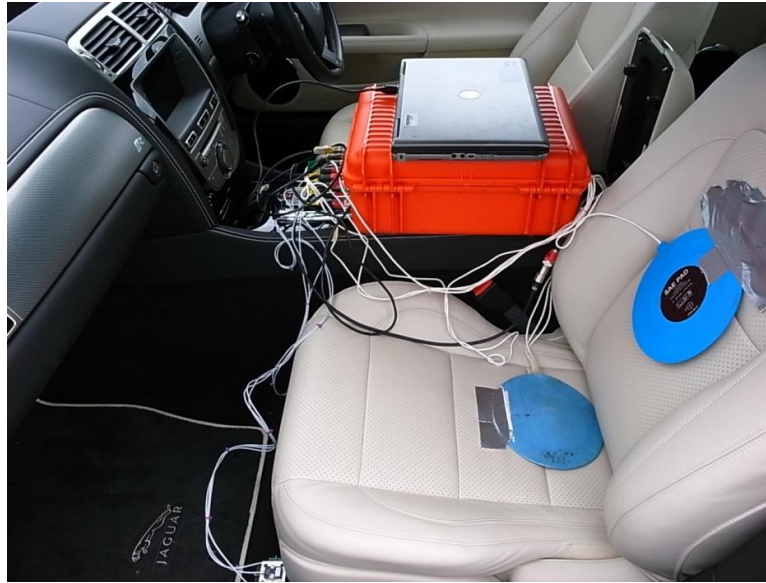
Figure 3.2 Accelerometers mounted on the front passenger seat.
