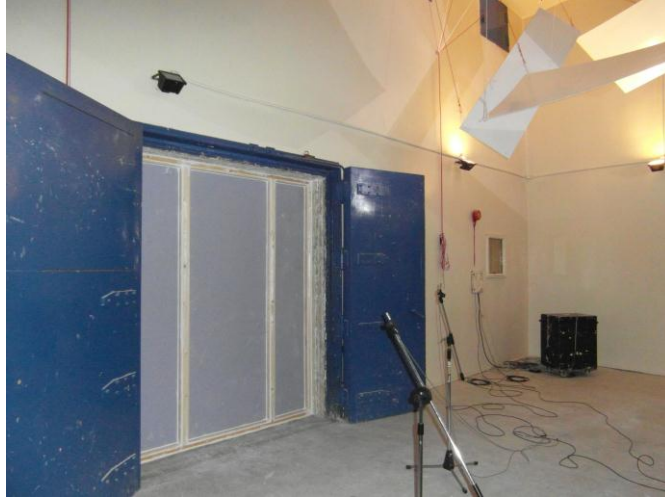
Figure 7.3. Measurement setup in the reverberation chamber
