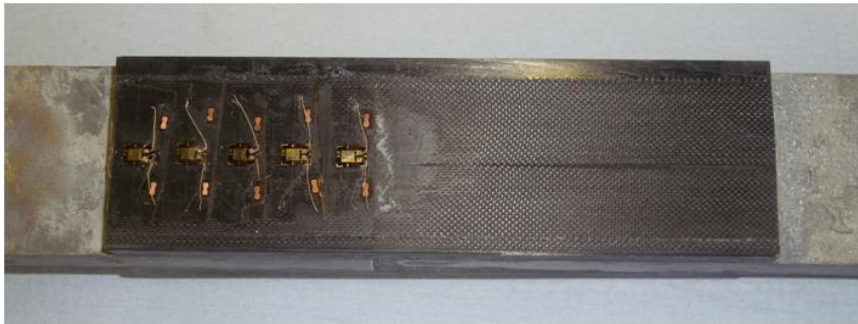
Figure 4.3: Strain gauges mounted on double-lap shear specimen
