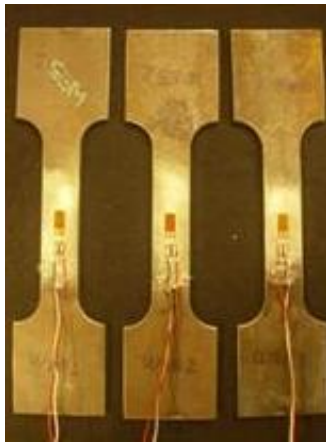
Figure 3.1: Strain gauges bonded on steel specimens
