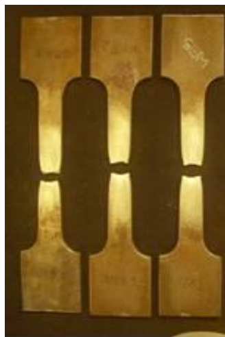
Figure 3.5: Fracture after necking in the middle of the steel dogbone tension specimens
