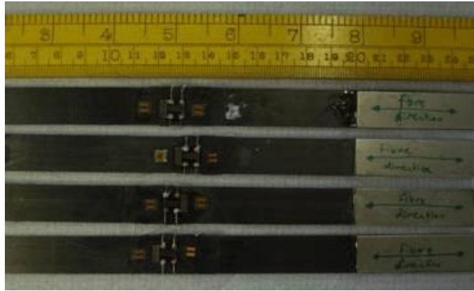
Figure 3.6: CFRP tension specimens with strain gauges and aluminium taps
