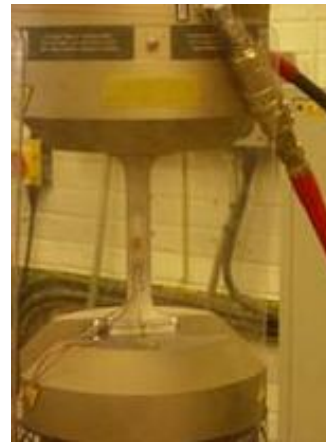
Figure 3.2: steel specimen loaded in tension
