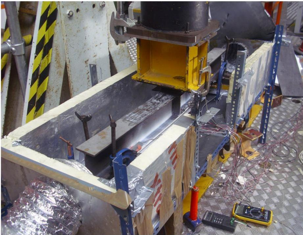
Figure 4.32: Specimen setup inside thermal chamber
