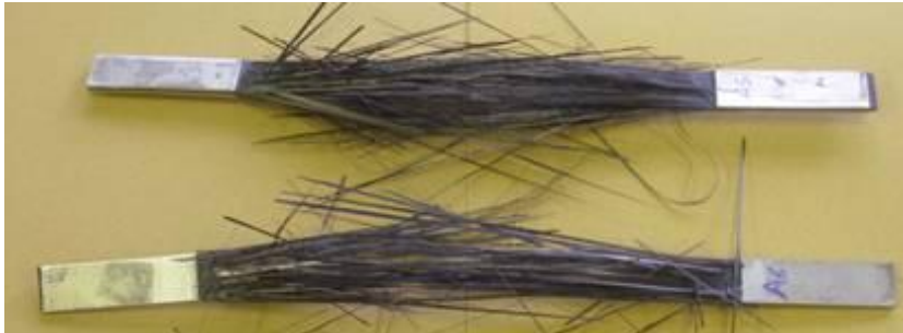
Figure 3.8: CFRP specimens after the tensile tests at 23 °C
