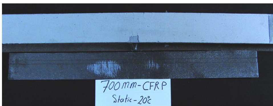
Figure 4.42: Failure mode of strengthened beams with different lengths of CFRP plate at 20 °C
