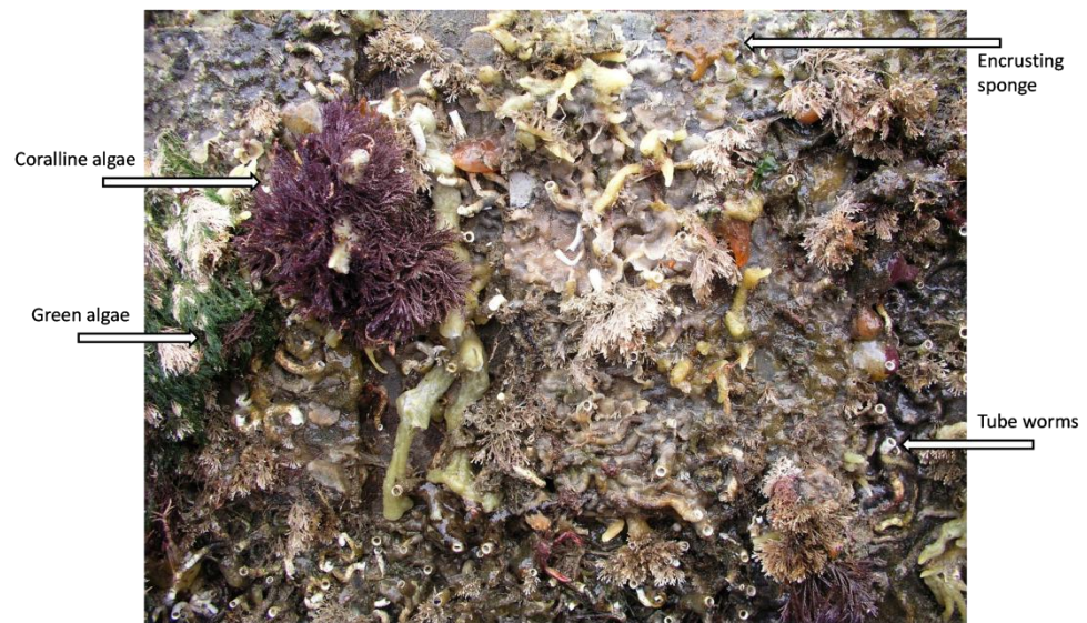
Figure 3.11 Wooden surface submersed in Southampton water, (UK) for 20 months with a complex biofouling community developed including coralline algae, tube worms, sponges, sea mats and sea weeds.
