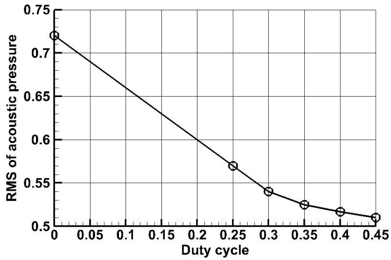
Figure 5.14: RMS of acoustic pressure in the far-field with duty cycle at AOA = 4 degrees, u_\infty = 25 m/s.
