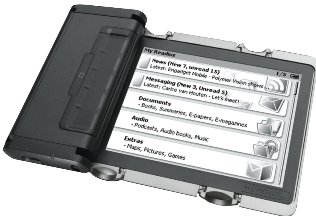
Figure 5.1: 'Readius' by Polymer Vision, using a display made on a rollable plastic film, enabling the screen size to be larger than the device body.
