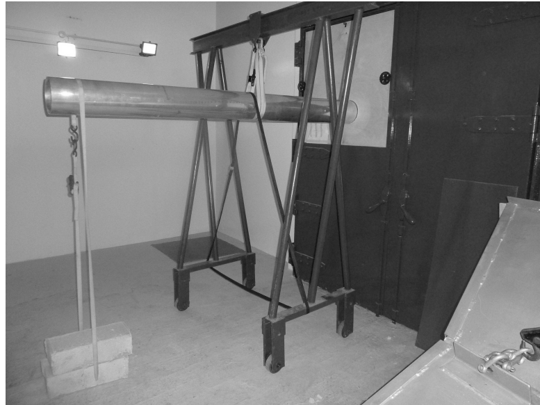
FIGURE 6.4: The reverberation chamber, with the nacelle duct leading into the University of Southampton's ISVR Large Anechoic Chamber.
