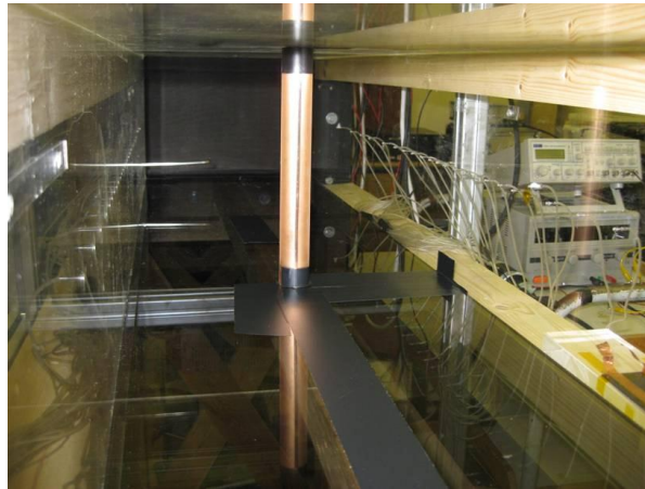
Figure 4.1: Cylinder model in the wind tunnel.
