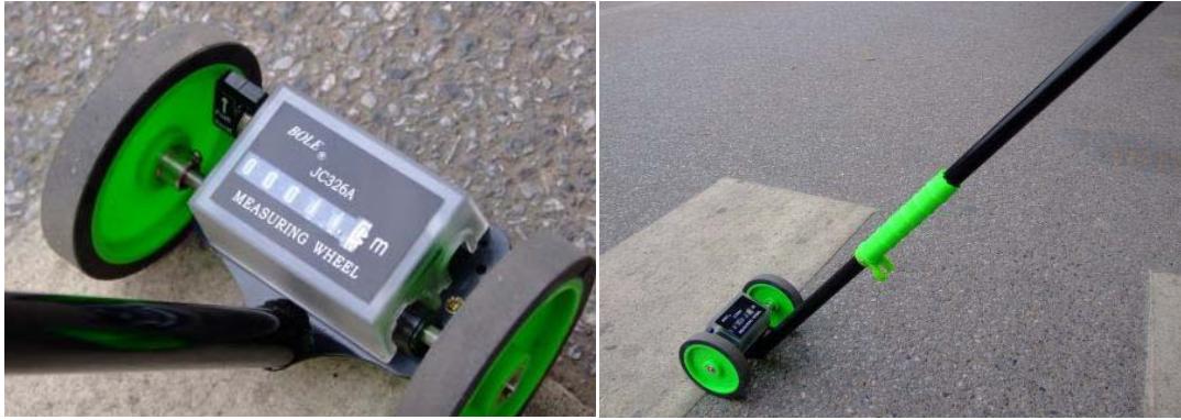
Figure 3.1 Survey of site characteristics using a measuring wheel
