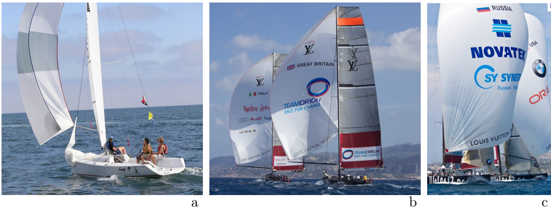
Figure 4.16: Different types of wrinkling arising on downwind sails. a: large amplitude wrinkles, b: singular wrinkle, producing a cusp; c: small amplitude wrinkles induced by the seams of the sail
