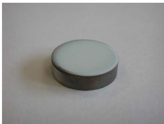
Figure 21 Typical Coated CMSX4 "Button" specimen (approximately 20mm x 5mm).
