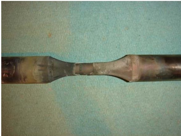
(a) Spallation of TBC in necked area
