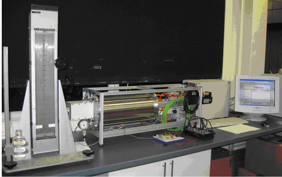
Figure 3.7 Pressure Sensor Circuit Connection and Calibration devices for Mechanical Lung rig (manometer in the left).
