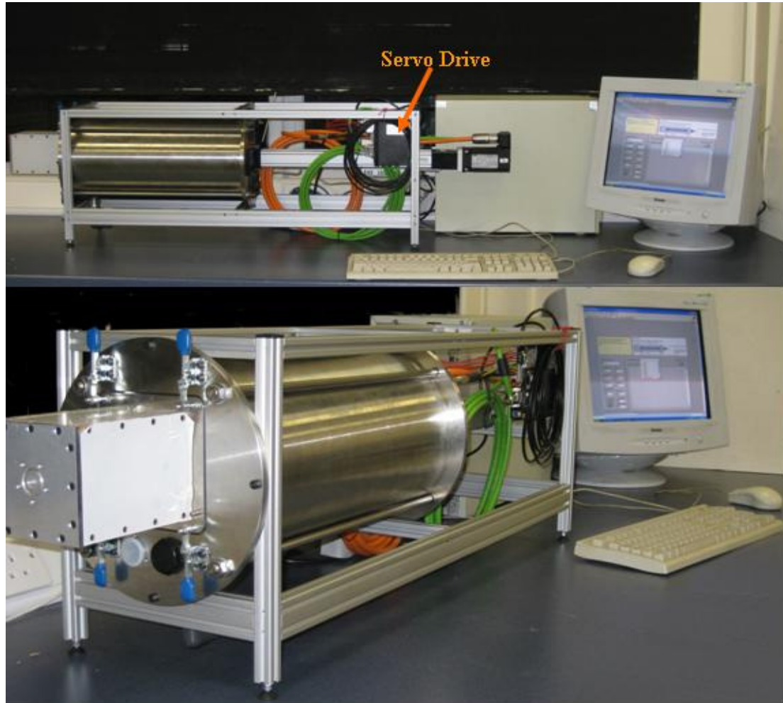
Figure 3.3 Mechanical Lung rig Rig assembly and connection to PC.
