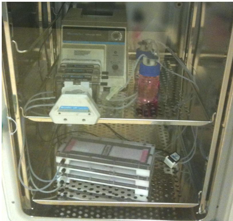
Figure 6.3 Pulsatile fluid flow (PFF) pumping configuration including peristaltic pump, media reservoir, tubing, flow probe and parallel plate device operating in a CO 2 incubator at 37°C and 5% CO 2 .
