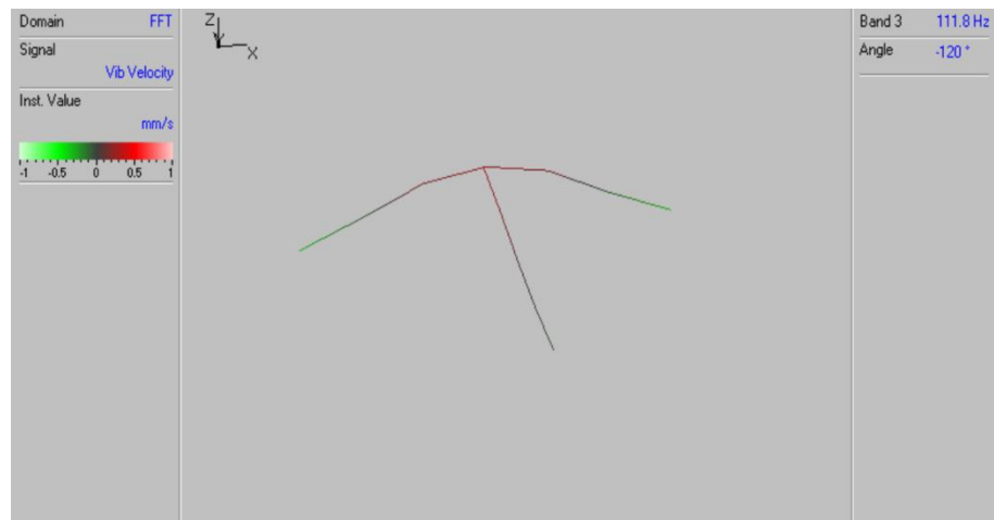
Figure 5.6: The first three operational deflection shapes (ODS) of the T beam configuration from laser vibrometer measurement when thin beam secondary beam was used. (a) First mode, flexural of the primary beam. (b) Second mode, twisted of the secondary beam. (c) Third mode, flexural of the secondary beam.
