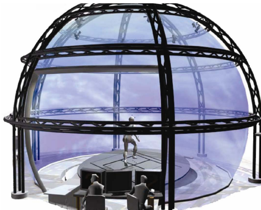
Figure 2.5: The CAREN: virtual reality system contained in a 7-m diameter dome with a six degree of freedom platform with a built-in instrumented treadmill (McAndrew et al. , 2010).
