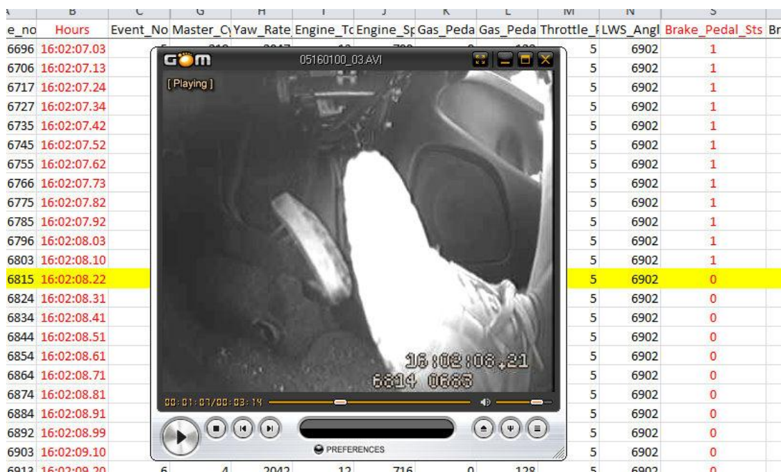
Figure 4-9: Brake pedal status and corresponding video image when brake was released
