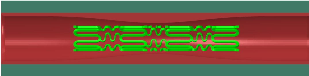
Figure 5.5: Assembly of the stent, plaque and artery (No balloon present)
