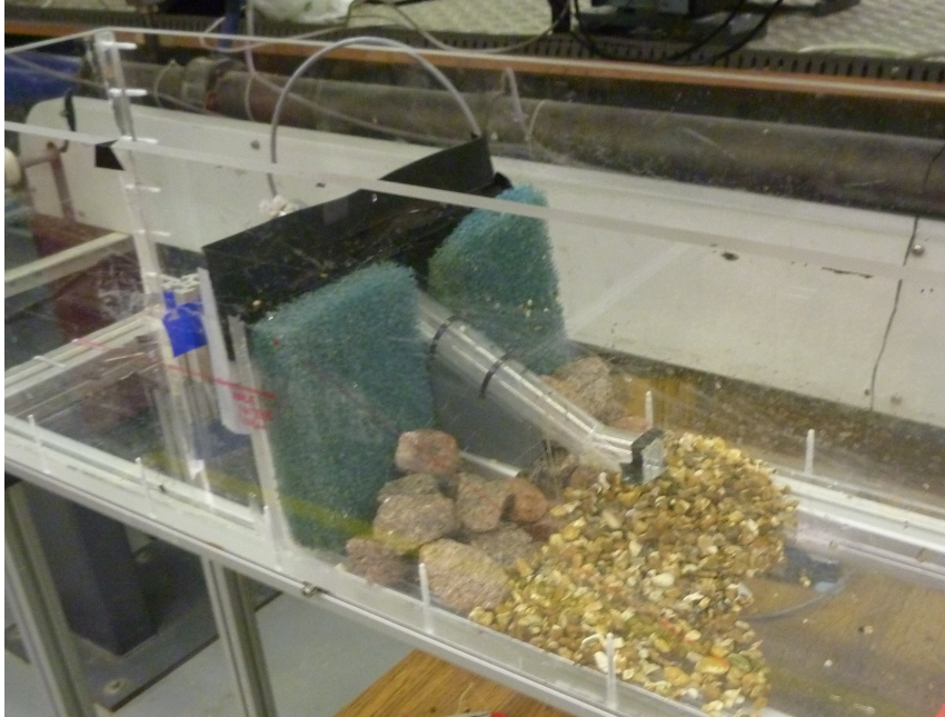
(a) Assembly of the rubble mound breakwater with installation of OWCP at the centre of wave flume within the structure
