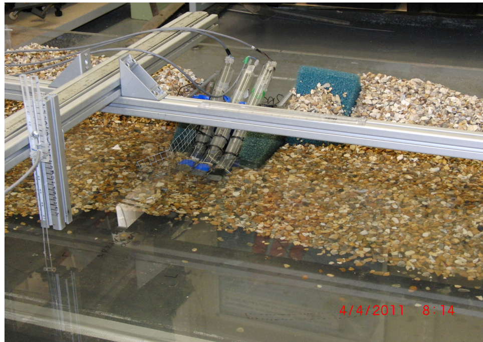
Figure 7.21: Installation of the 25-30-35 r array configuration within the 3D wave basin with s_d = 10 mm.
