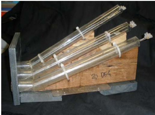
Figure 4: View of the 3 OWCPs array equipped with front reflective wall.
