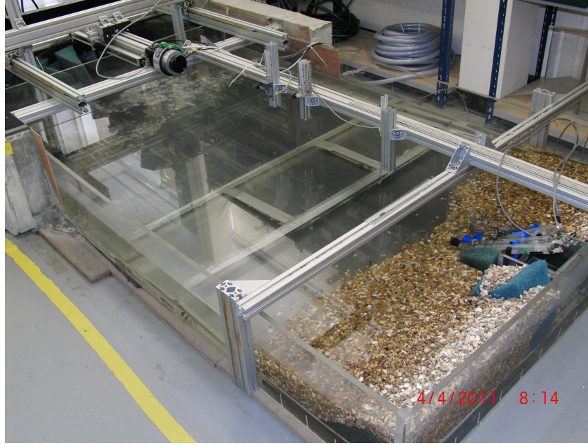
Figure 5.2: 3D Wave Basin equipped with linear wave generator and absorbing gravel beach.
