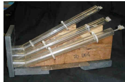
Figure 6 1:40 Model of 3 OWCPs organized in a closely spaced array
