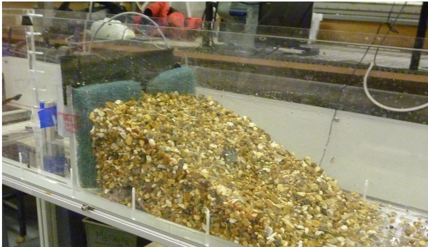
(b) Complete installation of OWCP the within the rubble mound breakwater
