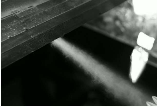
(c) Flow past a straight edge at 5° AoA.
