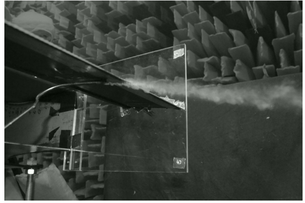
(b) Smoke wand on the pressure side of the airfoil.
