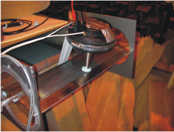
(a) Calibrator in-situ on the suction side of the airfoil.
