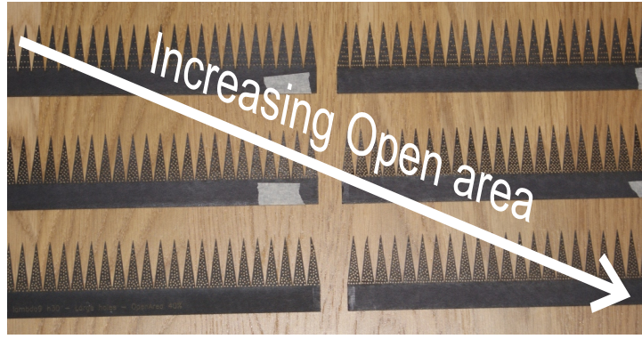
(b) Sawtooth trailing edges with holes cut in thick cardboard.
