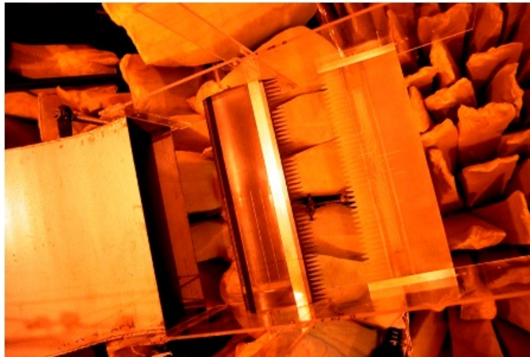
Figure 7.18: Fully treated tandem airfoils in the test section of the open jet wind tunnel.
