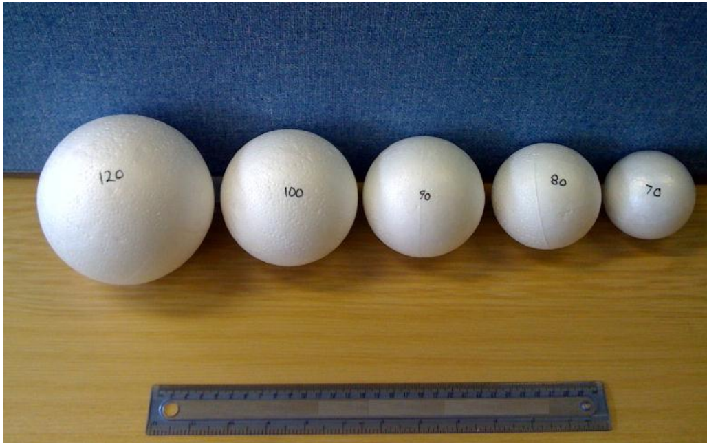
Figure 14: The five different sizes of polystyrene Styrofoam spheres used in the experiment. The numbers indicate the size of the diameter in millimetres. The ruler is there to represent the scale of the picture; it is 30 cm in length.
