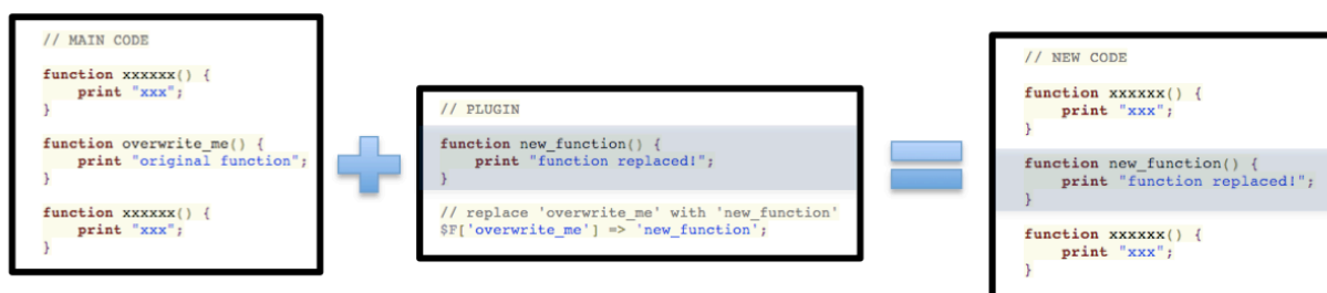
Figure 7 An example of function overriding
