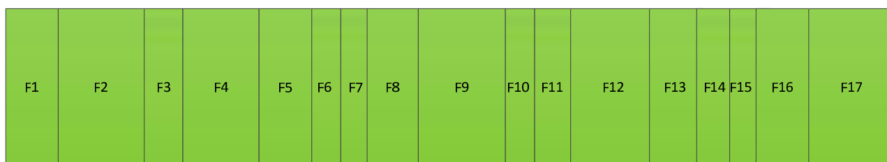
Figure 3 Representation of a set of files within a storage system. The files are labelled F1, F2 etc. The width of each file represents its file size.
