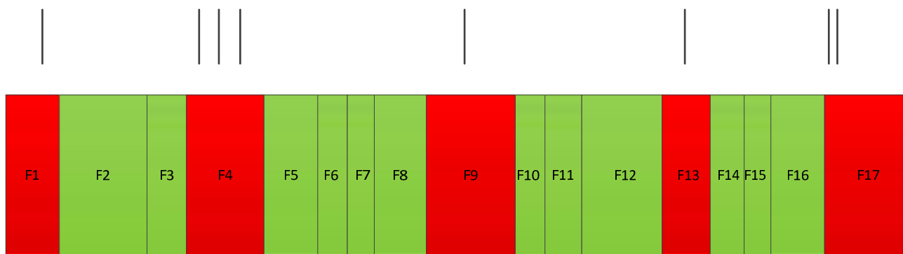
Figure 4 Example of bit level corruption (thin lines at top of the figure). Where one or more corruptions align with a file then the whole file is considered as corrupted (shown in red, e.g. F1, F4 etc).
