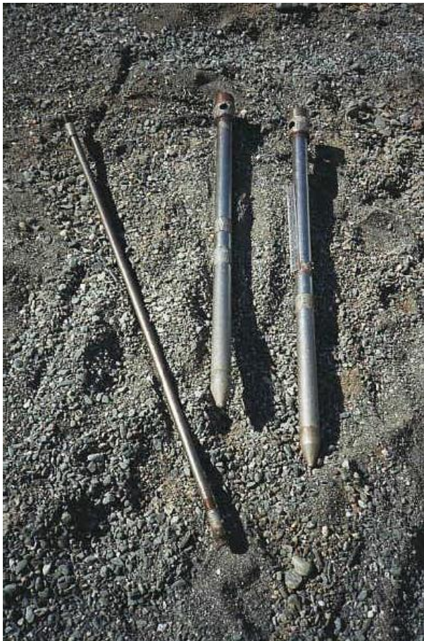
Figure 4.2. Example of the cores used to collect freeze core samples from cut and uncut redds (Evenson 2001).
