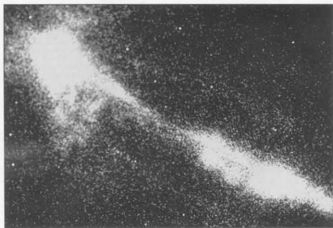
Fig 1 A photograph, taken through the image intensifier, of sonoluminescence in a 90% glycerine/10% water mixture, occurring within a cylindrically-symmetric sound field of 2 atm. pressure amplitude (see [4] for details). Each point of light represents the detection of a single photo. The bright sources of light arise from sonoluminescence from bubbles, originating from two regions. Connecting these is a string of bubbles, which may be luminescing or simply reflecting light from the main sources of sonoluminescence. The frame measures 11.75 mm x 17 mm.
