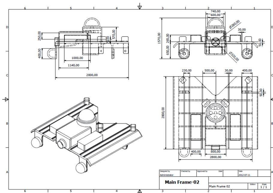
**Figure 3.14:** Design of main frame of the collector in terms of Design Phase II.
