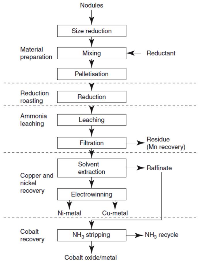
**Figure 3.27:** NML Process (Mukhopadhyay et al., 2008, Puvvada et al., 1997)
