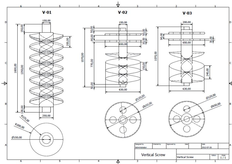
Figure 3.12: Designs of the vertical screw in terms of Design Phase III.
