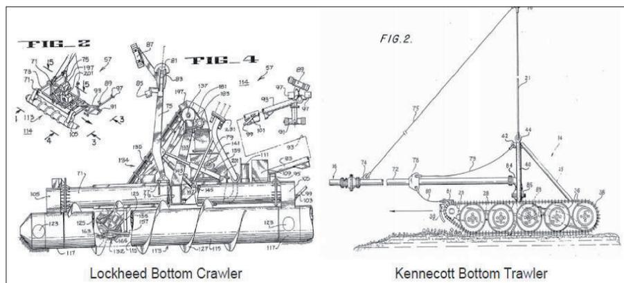
**Figure 2.2** Two different designs for nodule collectors as presented by Morgan. The Lockheed bottom Crawler is a self-propelled screw-based design (patented in 2011) whereas the Kennecott Bottom Trawler is a dragged track-based design.
