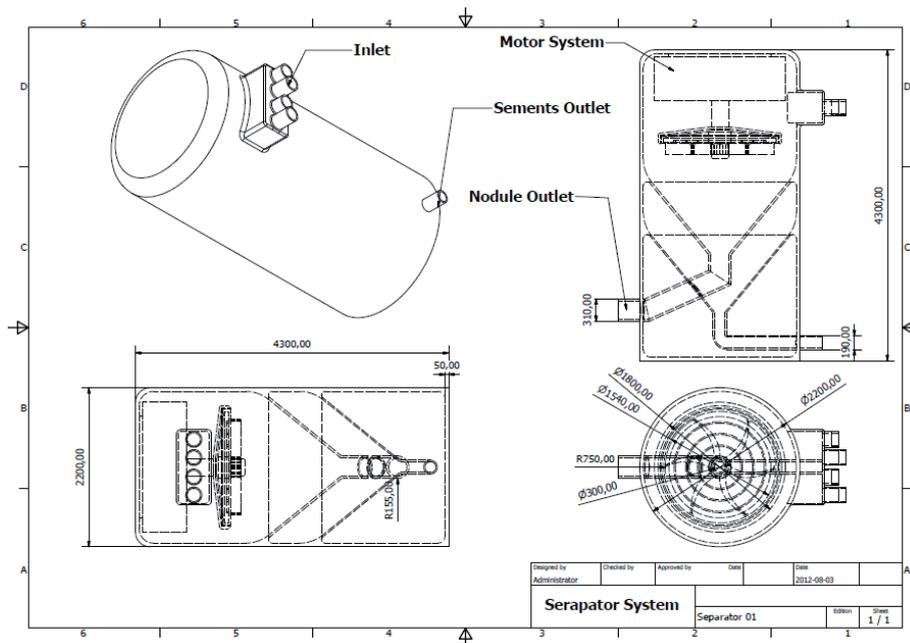
**Figure 3.20:** Design of the separation system.
