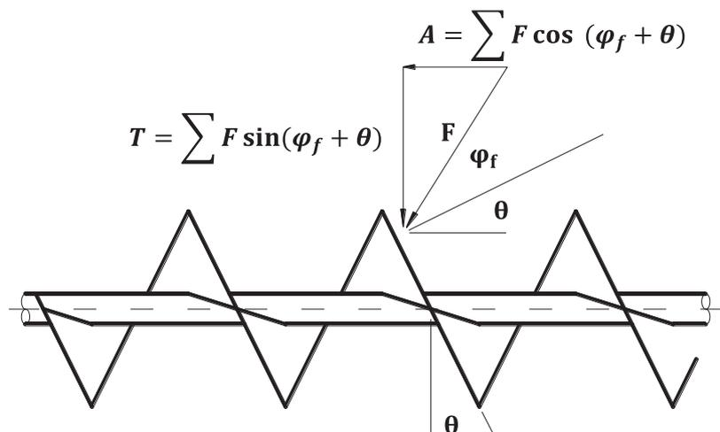
**Figure 3.9:** Force acting on the flight face
