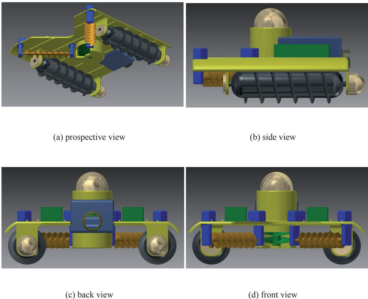
**Figure 3.6:** Conceptual design of the collector in design phase II.
