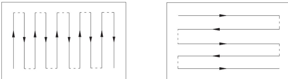
**Figure A.2:** Different Path direction for a rectangle area.
