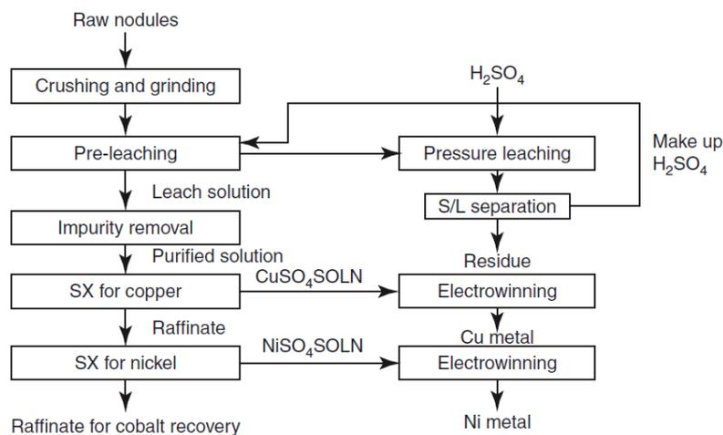
**Figure 3.31:** Sulfuric acid leach process adopted by Hindustan Zinc Limited (HZL) (Premchand and Jana, 1999).
