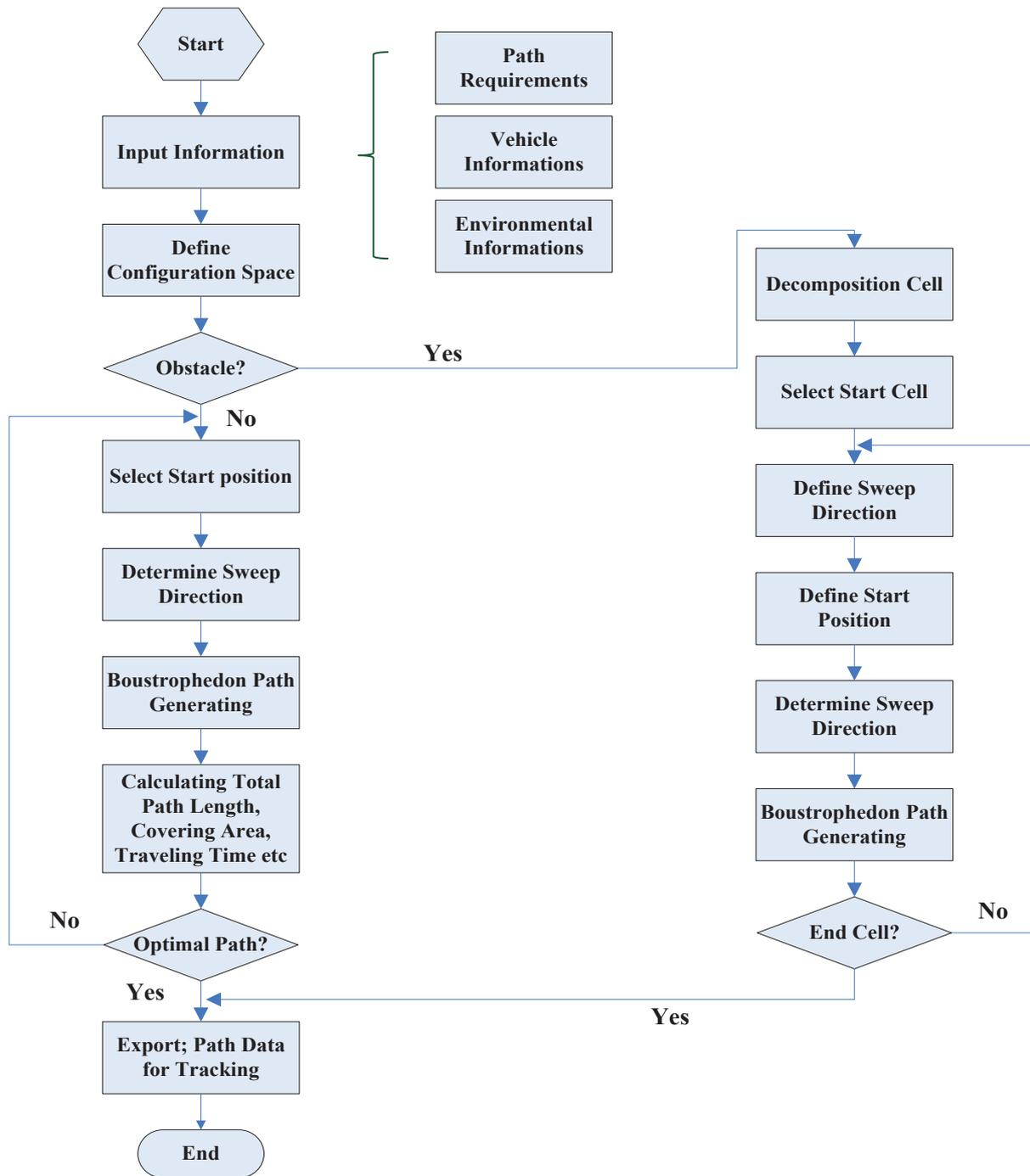
Figure A.6: Flow chart of collector sweeping method
