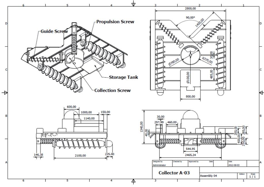
Figure 3.18: Design of the collector in terms of Design Phase III.
