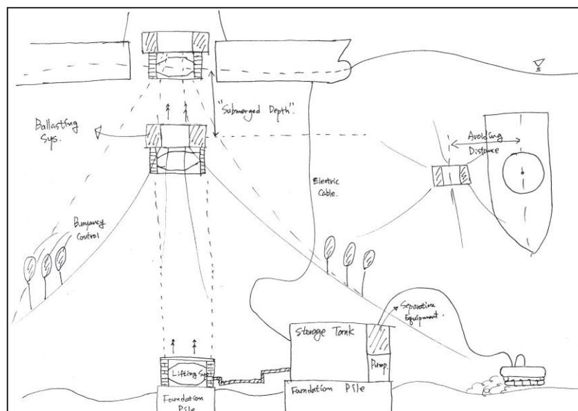
**Figure 3.40:** Container lifting system at the time of the HAZID
