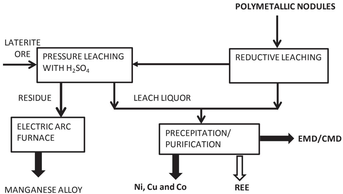
**Figure 3.42:** Metallurgical processing concept at the time of the HAZID
