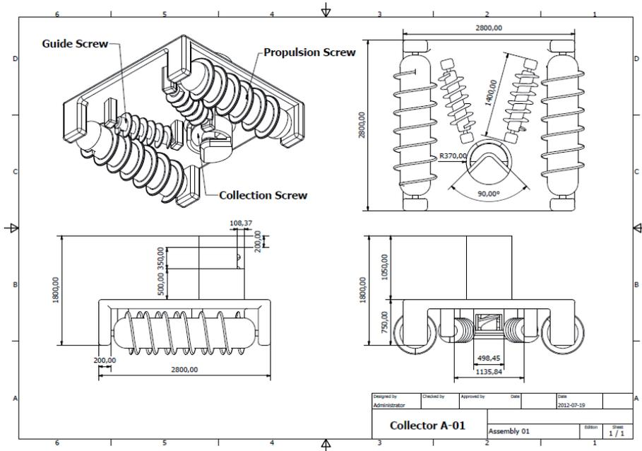
Figure 3.16: Design of the collector in terms of Design Phase I.
