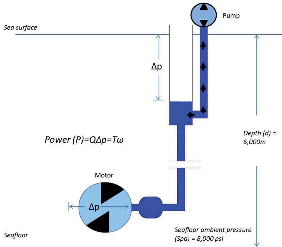
**Figure 3.37-** Subsea hydraulic power system.  $Q$ = flow rate  $T\omega$ = torque.
