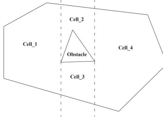
**Figure A.5:** Path direction decomposed while there is an obstacle
