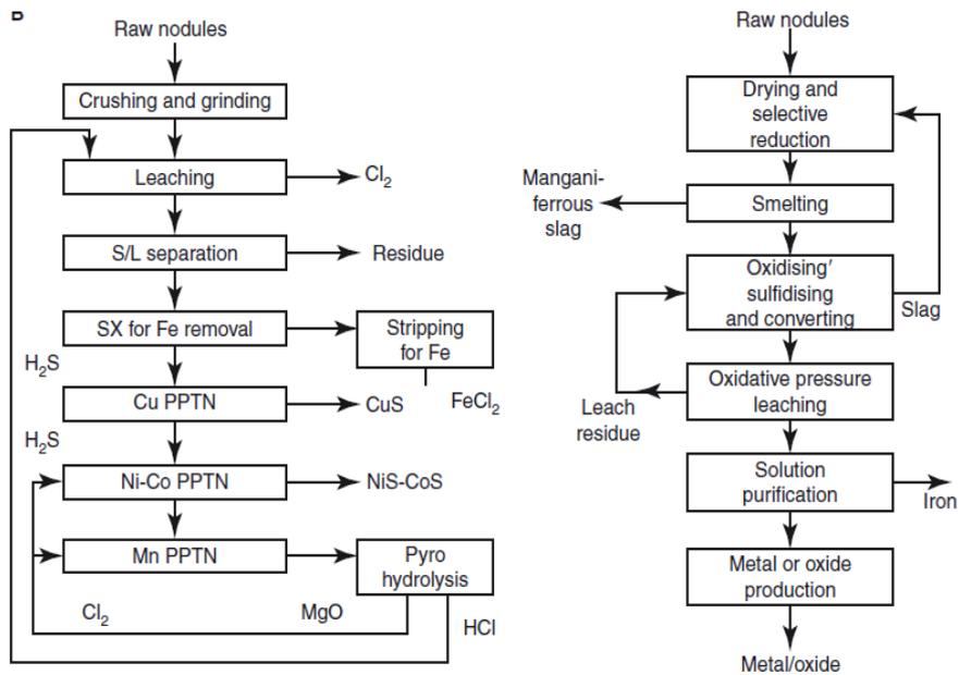
**Figure 3.34** MHO hydrochloric acid leach Process (left) (Van Peteghem, 1977) and INCO Process for smelting and sulphuric acid leach (right) (Sridhar et al., 1976).
