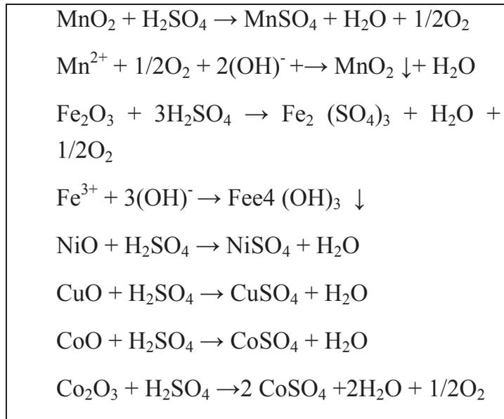
**Figure 3.30:** High Temperature and high pressure sulfuric acid leach reactions (Haynes et al., 1985)
