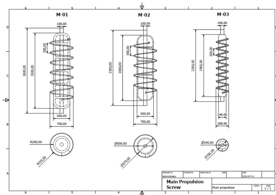
**Figure 3.10:** Designs of the main propulsion screw in terms of design phase I.
