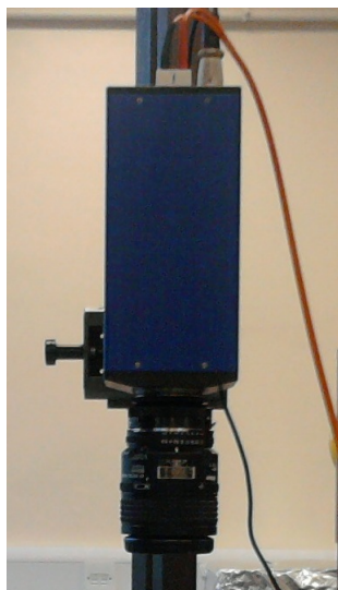
Figure 4.3: Nikon AF Micro-Nikkor lens 60 mm f/2.8D mounted to the CCD camera.
