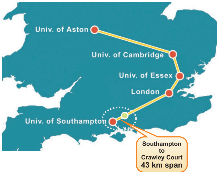
Figure 6.3: The JANET-Aurora network is a dark fibre network linking four universities in the south of England over a total span of over 800 km. Two fibres are available on each the span between universities. A number of hubs are present between major spans. The comb transfer experiment described in this chapter was carried out on the first span from the University of Southampton to a hub in Crawley Court located 43 km away. The two fibres were joined together at the hub in order to create a loop where both the transmitter and receiver (user) ends are in the laboratory at the University of Southampton.
