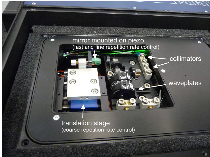
Figure 4.18: Photograph of the NPL Menlo Systems fibre laser module with the lid removed. The free space optics is required to achieve a wide tuning range of the repetition rate. The waveplates complement the computer-controlled squeezers in order to allow all possible polarization states to be obtained.
