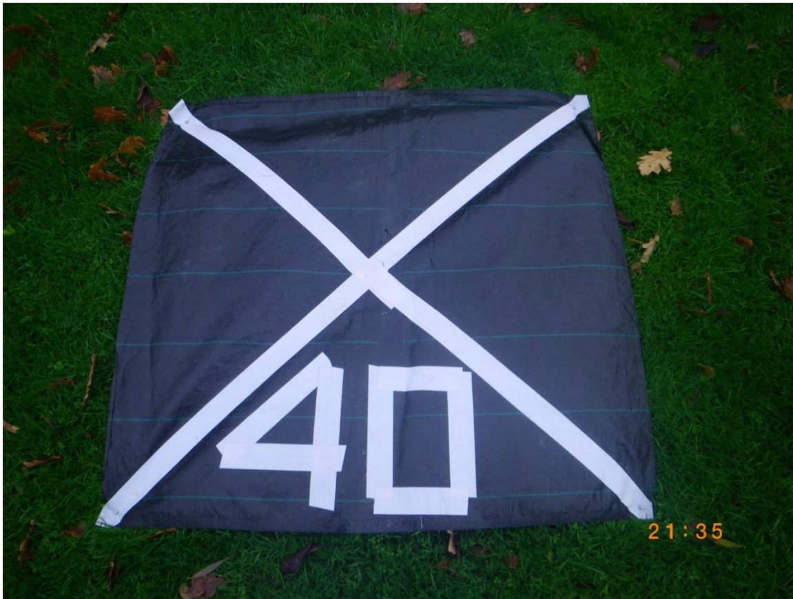
Figure 7.32. An aerial photography target. Targets were held in place by a four three inch nails, one in each corner.
