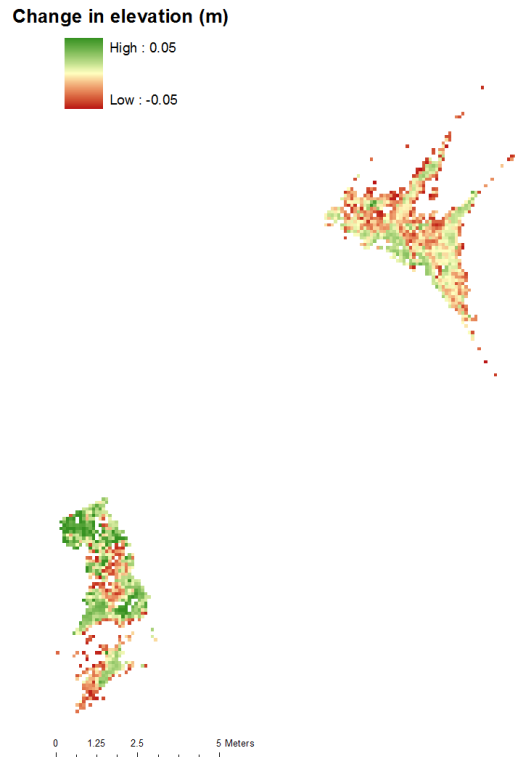
Figure 7.18. Digital elevation model showing changes in river bank elevation between 22/03/11 and 13/05/11 at the Southern Midlington site.
