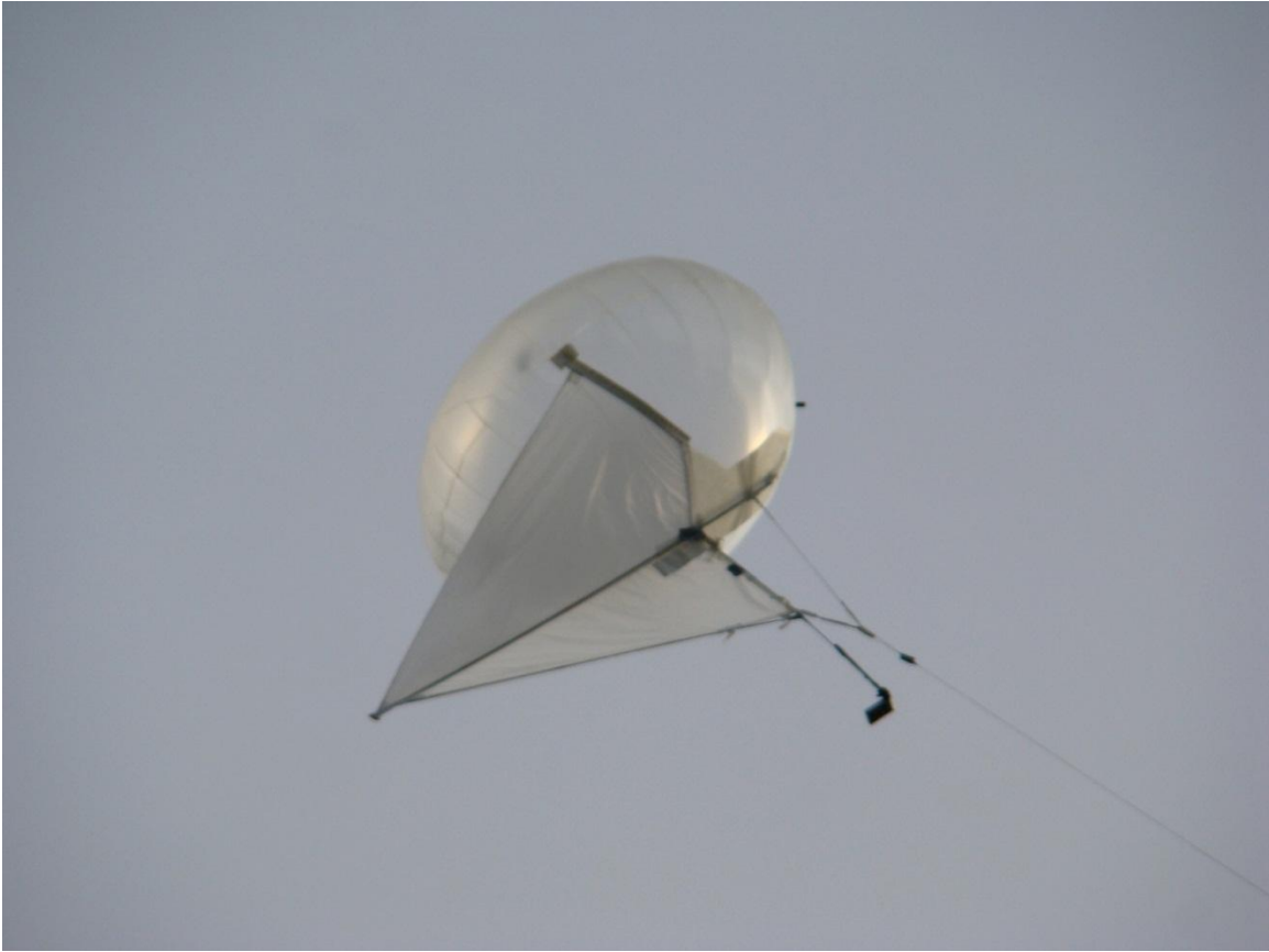
Figure 7.31. The aerial blimp and kite with camera attached and trailing line visible (Photo courtesy of Simon Dixon)
