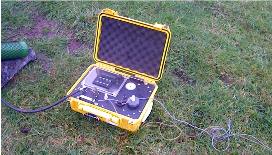
Figure 7.6. The cohesive strength meter in the field.
