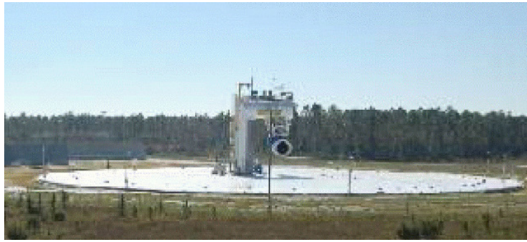
FIGURE 4.13: Experimental set-up for static noise test for a HBR turbofan engine
