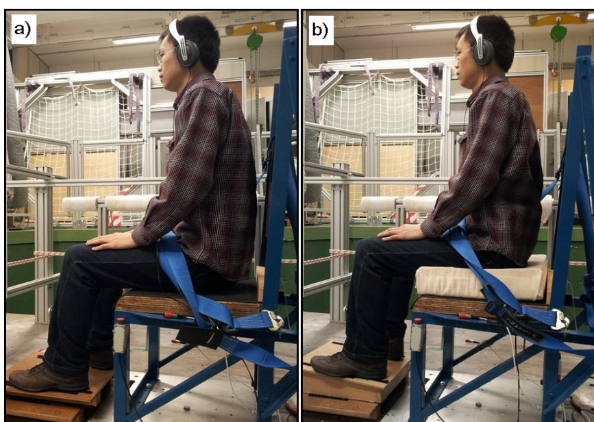
Figure 7.1 Illustration of the two seat-pan conditions (a) rigid seat; (b) foam cushion.
