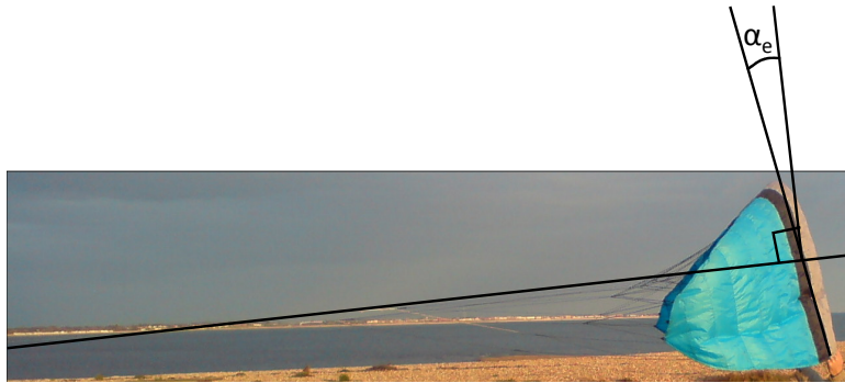
Figure 3.4 Illustration of measurement of built-in angle of attack
