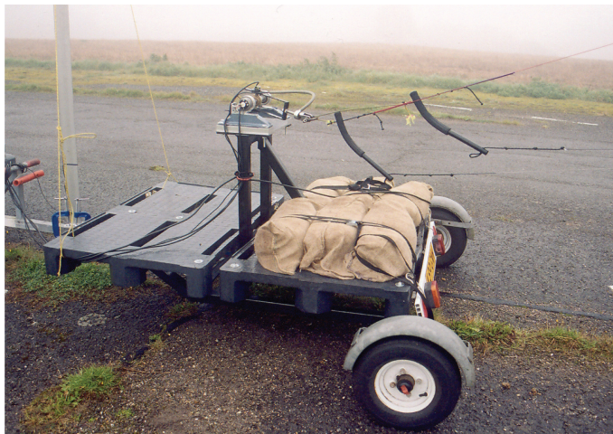
Figure 2.3 The towed dynamometer trailer
