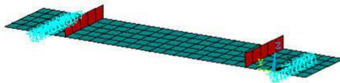
Figure 37. FEM of the CFRP samples, showing supports (pale blue) and masses (red).
