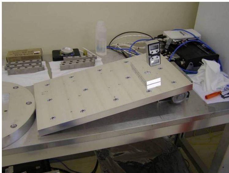
Figure 77. Static friction measurement setup
