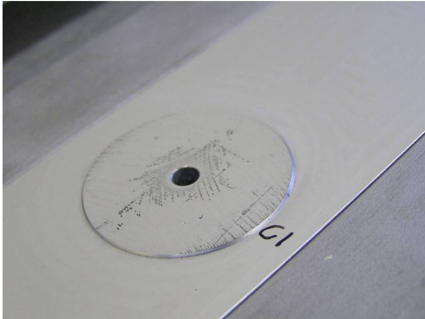
Figure 85. Blackening of joint observed following testing.
