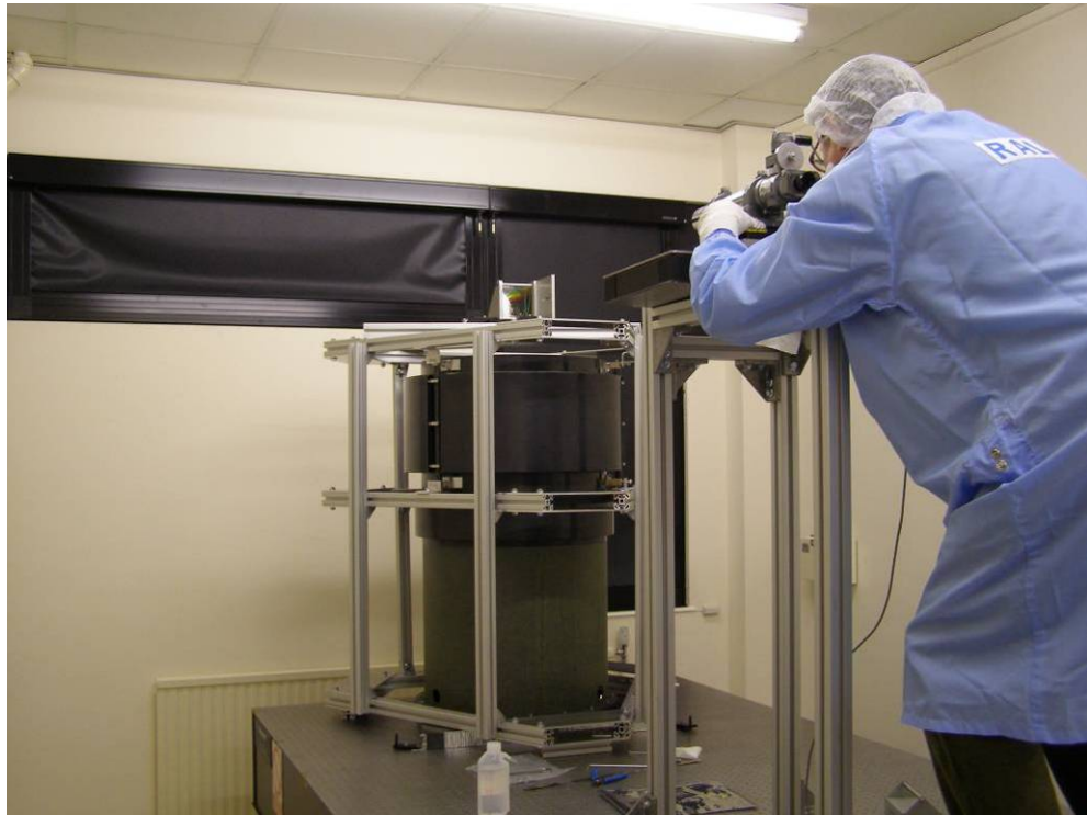
Figure 14. Using autocollimator to check alignment for gravity sag test.
