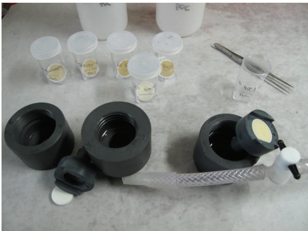
Figure A.4: Filter holders used at sea for the filtration of the thorium small volume technique.
