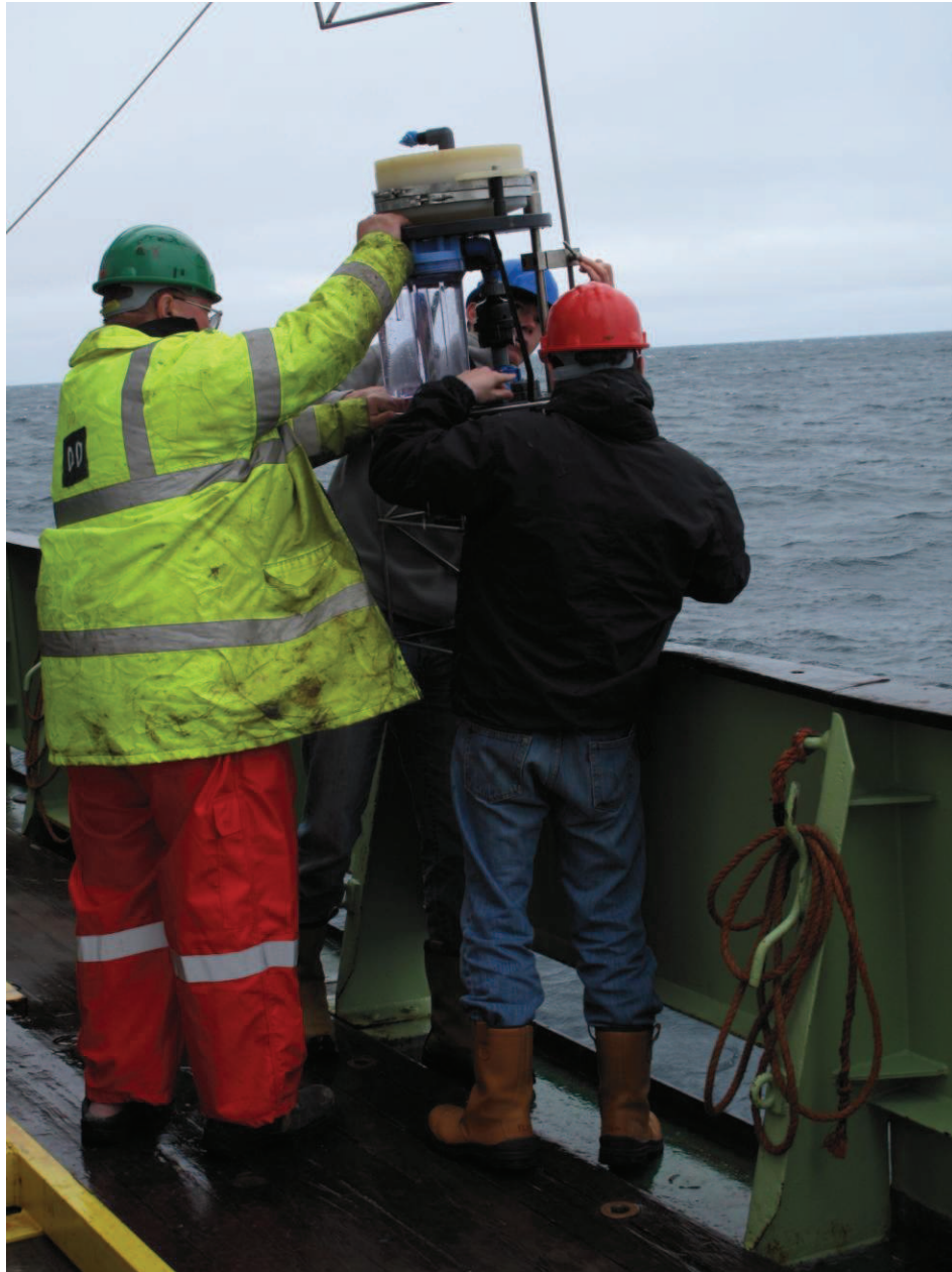
Figure A.6: SAPS deployment during D354 onboard the R.R.S. Discovery with help of Chris Marsay (University of Southampton) and “DD” (NMF).
