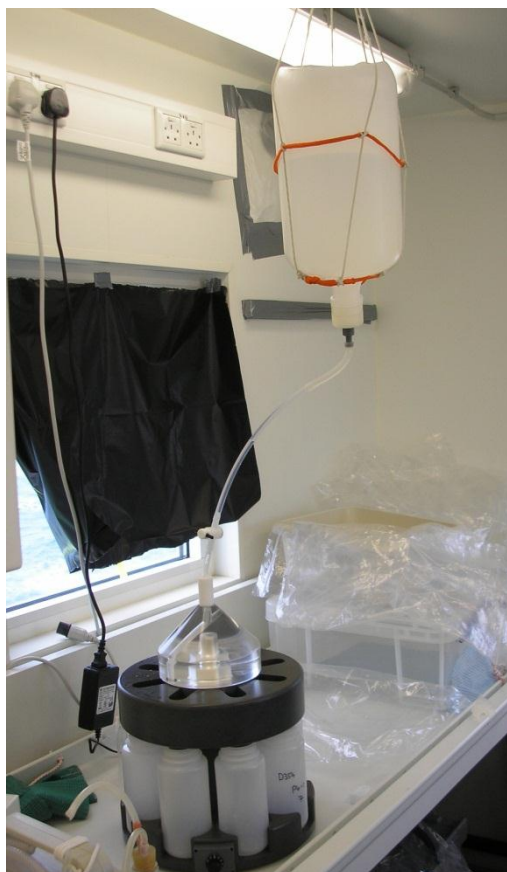
Figure A.2: Set-up used to split PELAGRA samples, showing the 4 L bottle into which cups were combined (inverted in photo) and the rotary splitter, loaded with 500 mL bottles.
