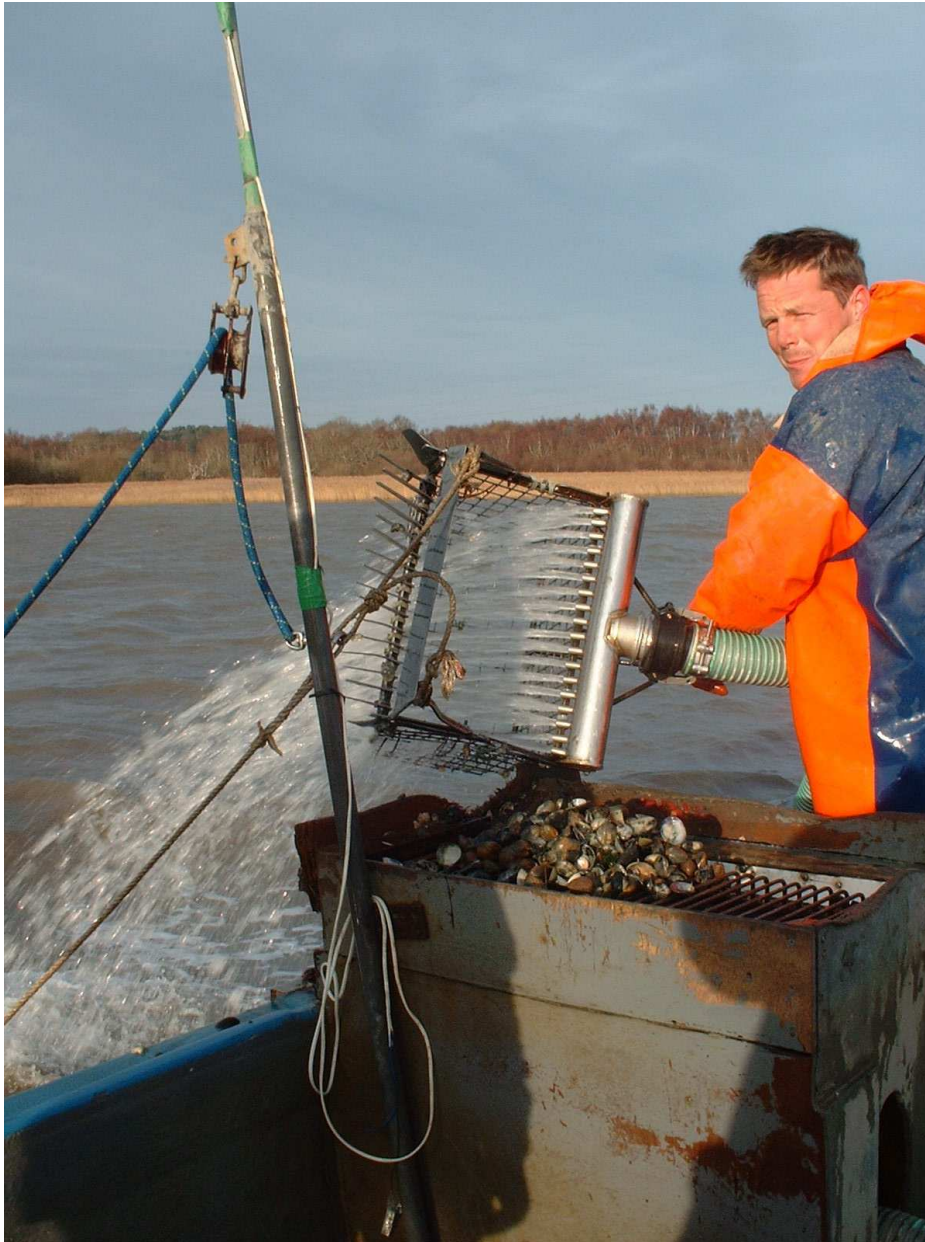
Figure 3 The 'pump scoop' for harvesting T. philippinarum in Poole Harbour (Figure courtesy of Dr. Antony C. Jensen)
