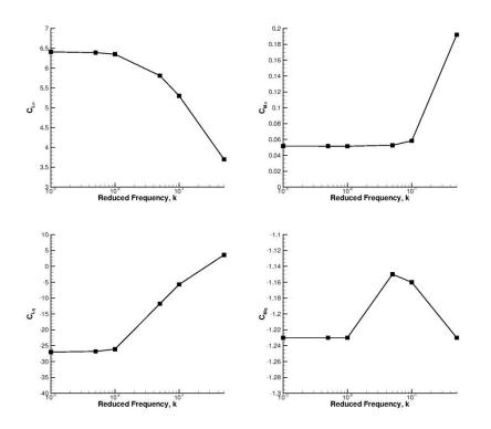
Figure 10: Variation of dynamic derivatives with reduced frequency
