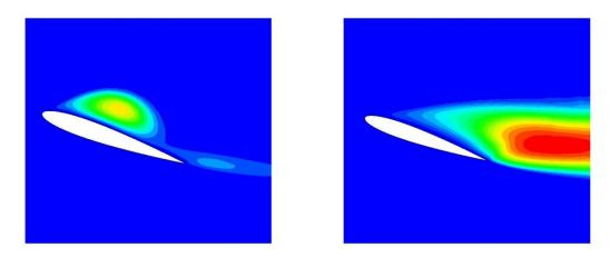
Figure 6: Turbulent nu term at 19.24 degrees on the upstroke (left: unsteady, right: quasi steady)
