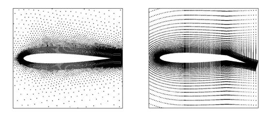
Figure 1: Aerofoil clouds (left: RANS cloud, right: Euler cloud with flap at 15 degrees deflection)
