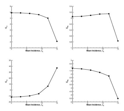
Figure 8: Variation of dynamic derivatives with mean incidence
