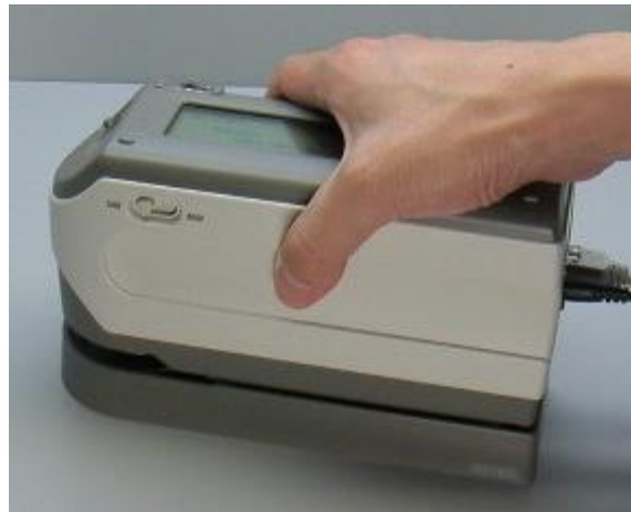
Figure 10: An example of a modern scanning spectrophotometer, the Konica-Minolta CM2600-d.
