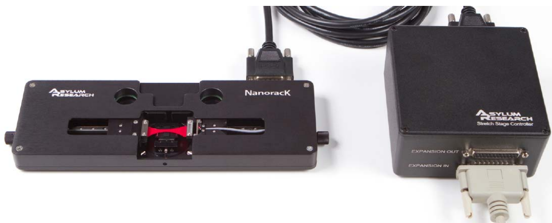
Figure 3-5: (a) The nanorack ® stage. The tensile stage is carried on the MFP-3D's XY scanner and interfaces with an instrument box containing signal conditioning electronics that are SmartStart bus compatible. The dual axis position encoders provide 5 \mu\text{m} positioning accuracy over the full 6 cm range of travel (12cm total) (Image courtesy of Asylum Research)
