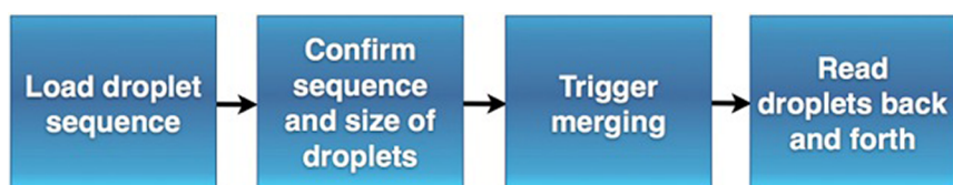
Figure 4. The automated workflow programmed to run kinetic assays. Schematic diagram of the four steps that provide a full set of Michaelis–Menten data: (1) loading of the droplet pairs corresponding to different points of the Michaelis–Menten plot; (2) confirming and sizing of the droplet pairs prior to fusion; (3) droplet merging in tubing initiates the reaction; and (4) droplets are moved back and forth for reading of the reaction progress by absorbance. Such readings can be repeated many times until the reaction has advanced sufficiently to describe a full time-course. The ability to carry out as many measurements as necessary makes this system amenable to most reactions (with time scales from a minute to several hours or more). The sizing data (step 2) and the data for the time-courses (step 4) were stored in individual files. This process can be repeated for multiple samples that are sequentially supplied from the carousel of the robotic sampler (Figure 1A).
