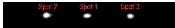
Figure 7.7.1 The modal image pattern of the 1x3 MMI device recorded by the NIR camera at 1641 nm.
