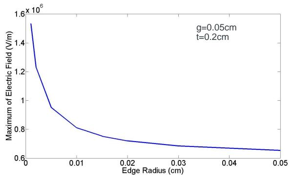
• When the distance between the upper and lower electrode and the distance between guard and measuring electrode is constant, a larger edge radius will result in a lower electric field.
