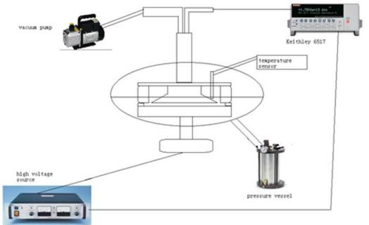
The test system includes the test cell, a HV power supply, a vacuum pump, a Pico-ammeter and a fan-assisted oven.
