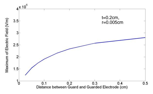
• When the distance between the upper and lower electrode and the edge radius is constant, a larger distance between the guard and measuring electrode will result in a higher electric field.
