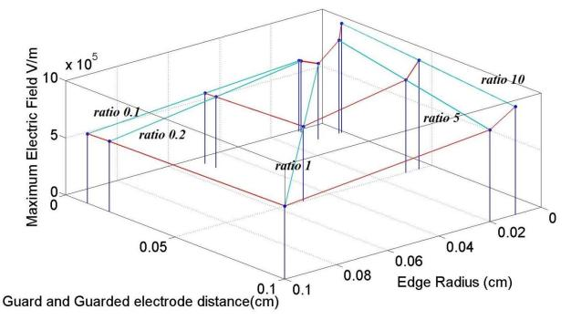
If assuming the distance between upper and lower electrode is far larger than the gap distance and radius, it is obvious that it is the ratio of the distance between the guard and guarded electrode and the edge radius that determines the maximum electric field in the oil test cell. For a further recommendation, this ratio should never surpass 1.
