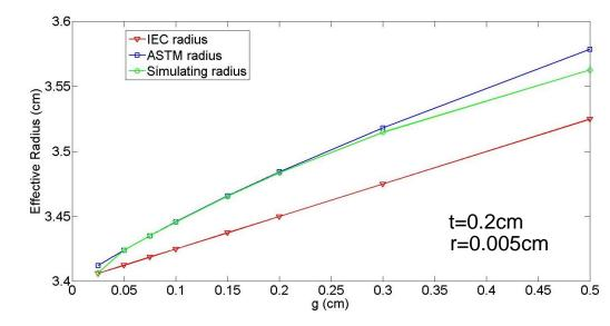
• When the distance between the high voltage electrode and measuring electrode and the edge radius are constant, the calculated the effective measuring electrode radius is close to the value calculated from ASTM standard. However, the difference between the radius calculated from the current standards is not significant.
