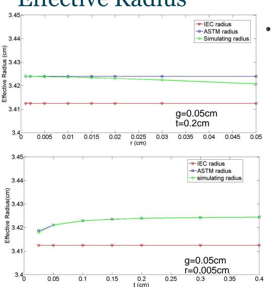
• As seen from the simulating result, the effective radius calculated from simulation is close to the value calculated according to the ASTM standard and a little higher than that obtained from the IEC standard. The difference between the radius calculated from those two standards are not notable.
