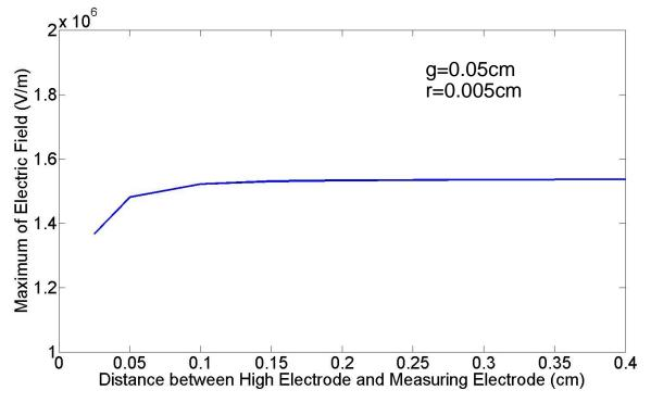
• When the edge radius and the distance between guard and measuring electrode is constant, a larger distance between the high voltage electrode and measuring electrode will result in a higher electric field.
