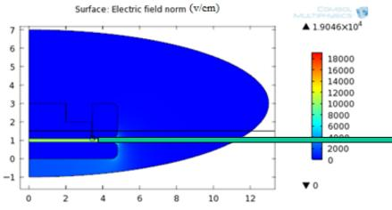
Here, we set the gap between upper and lower electrode is 0.2cm, the distance between guard and guarded electrode is 0.05cm, edge radius is 0.005cm and the applied voltage is 2000V
