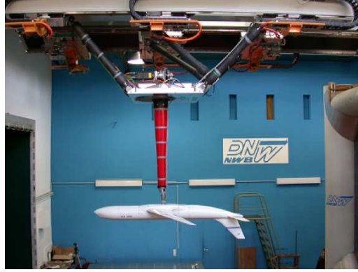
Figure A.8: Wind-tunnel testings of the DLR-F12 model in DNW-NWB [200]
