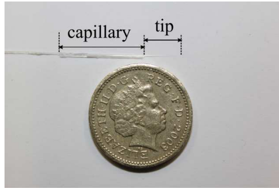
Figure 4-3 Picture of a MFCT. The capillary has 600 \mu\text{m} inner diameter.
