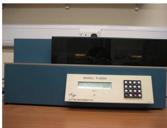
Figure 1-7 Picture of P-2000 micropipette puller (SUTTER INSTRUMENT Inc., Novato, USA).
