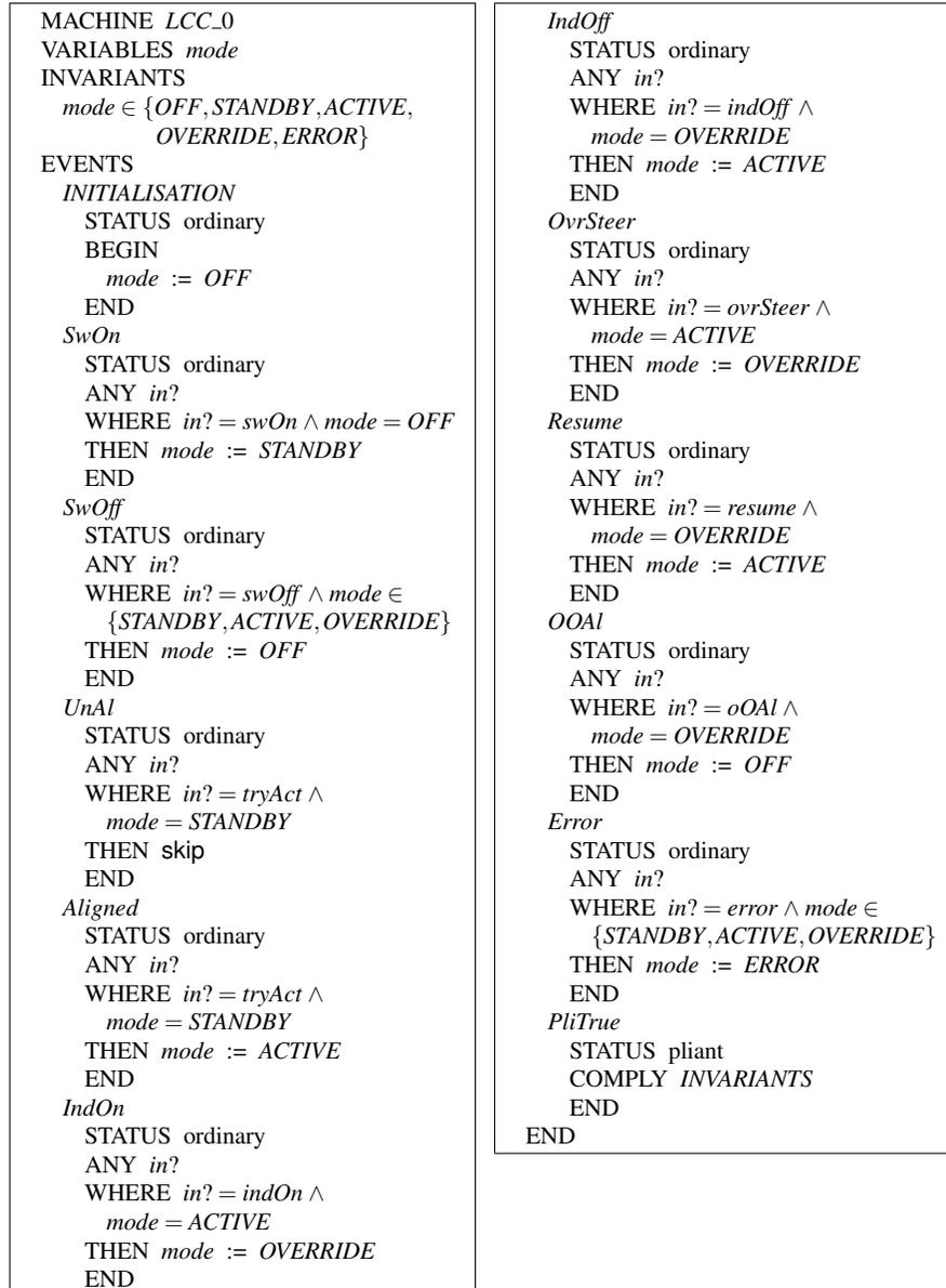
**Fig. 3** Mode level description of lane centering control.
