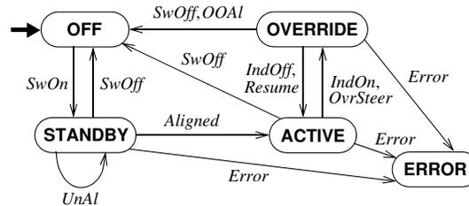
**Fig. 2** The state transition diagram for a simplified LCC.
