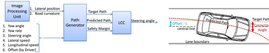
**Fig. 1** Architecture of a lane centering controller (LCC) on the left. On the right, a schematic illustration of the geometric elements that figure in LCC computations.
