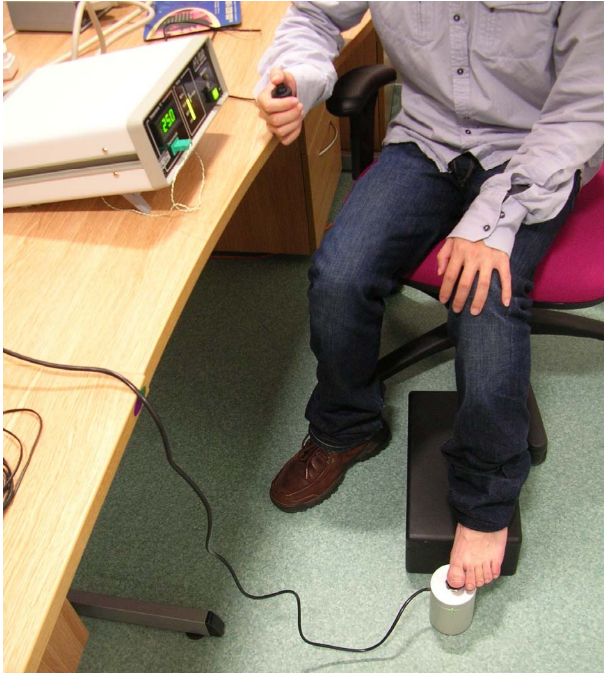
Figure 1 Posture of a subject during the measurement of vibrotactile thresholds at the big toe with HVLab Vibrotactile Perception Meter (VPM).
